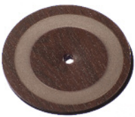
HOT STAMP FOIL - TOTAL LOSS OF FOIL - WEAR INTO SUBSTRATE
